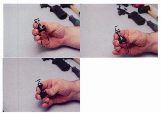
4. Insert the hammer assembly into the receiver and secure it with a retaining pin. Insert the assembled trigger group and secure it with a retaining pin. Be sure that all the parts are assembled and look like the pictures above. Once everything is in place, secure it all with a retaining plate or spring (A).
