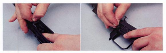
5. Insert the selector lever (A). With pliers, remove the hammer spring legs, placing them on the end of the trigger (B). The hammer will need to be pushed down until it engages with the trigger to allow the bolt to be inserted (C). Reinstall the bolt, recoil spring, and cover. With no ammunition in or around the weapon, dry fire the weapon several times in a safe direction to ensure a successful installation.
